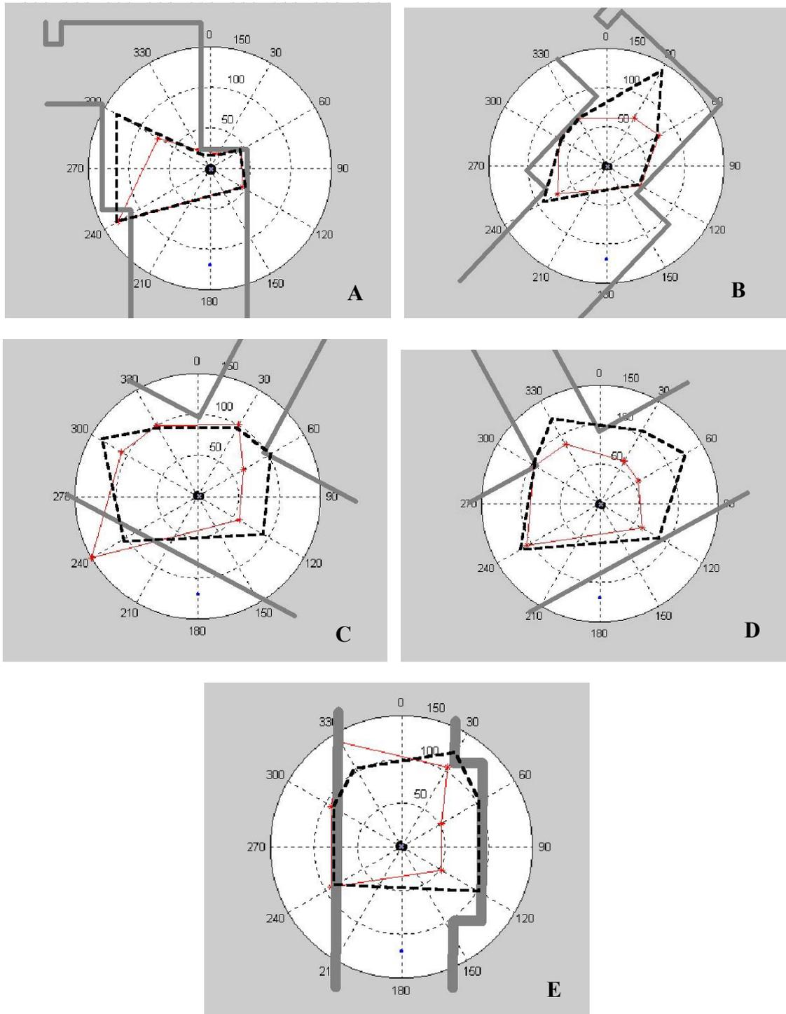
**Figure 6.** Omni-directional range measurement results for 5 different indoor scenarios (A – E). The thick and continuous gray lines represent wall boundaries in the test environment. The thick dotted lines represent range measurements acquired with the Sweep mode. The thin continuous lines represent range measurements acquired with the Flood mode. The three concentric circles represent 50-, 100- and 150-inch ranges.
