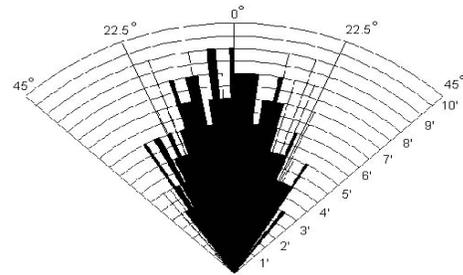
Figure 4. Beam pattern for the Devantech SRF04 sonar
