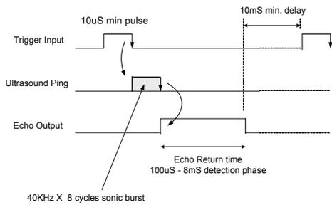
Figure 3. Timing diagram for the Devantech SRF04
