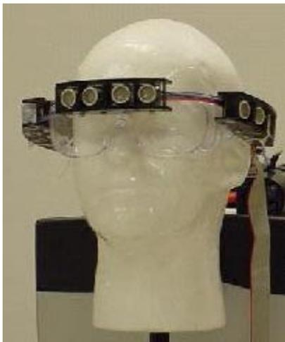
**Figure 1.** Headgear housing the six sonar modules
