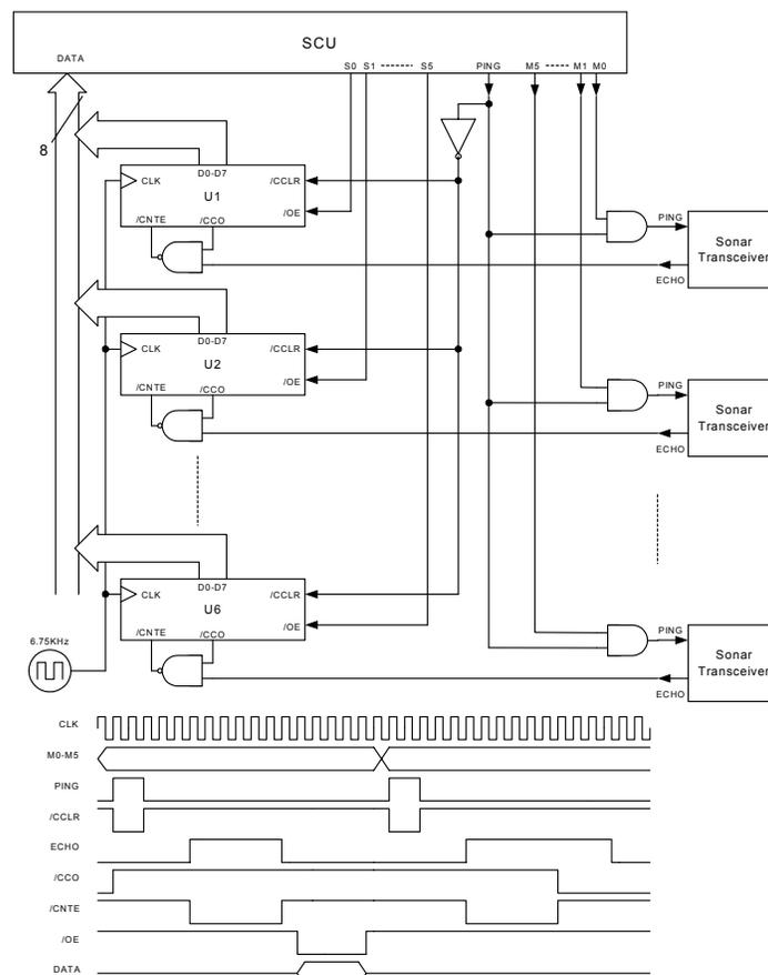
Figure 5. SCU schematic and timing diagram describing the sonar module interface technique
