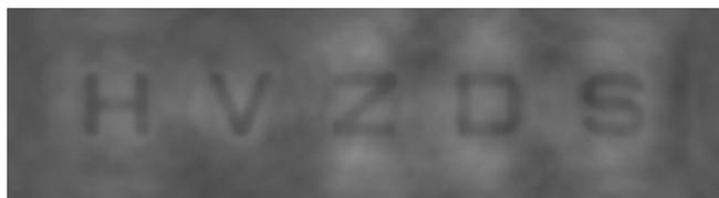
Figure 6- Simulated image of what the person would see when viewing Figure 3 through the -6.0 diopter lens.
