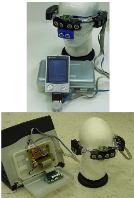
Figure 10. Photograph of the fully constructed prototypes: The Pocket PC based system (top) and its precursor, a laptop PC based system (bottom). The photographs show the host computer, SCU and the sensor array.
