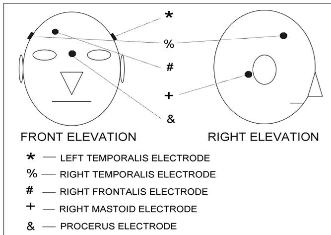
Fig. 2. Electrode placement diagram for EMG system
