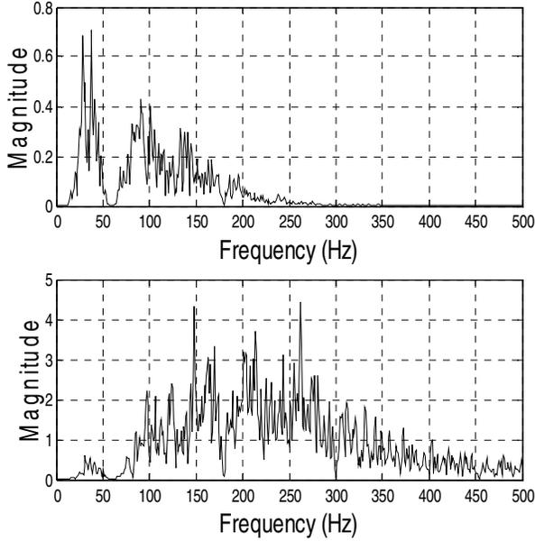
Fig. 1. Spectra observed during a right frontalis contraction (top plot) and left temporalis contraction (bottom plot)
