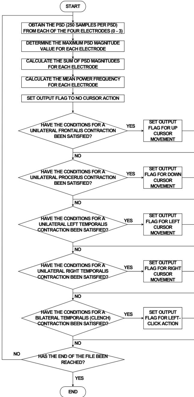
Fig. 4. Flowchart of EMG-based classification algorithm
