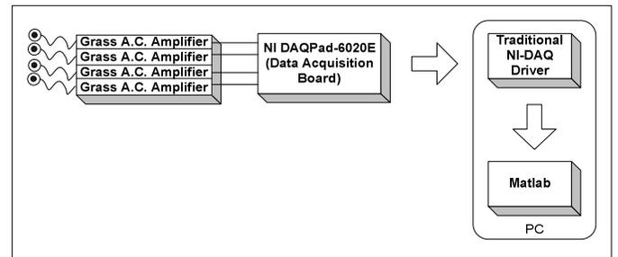
Fig. 3. Recording Structure for EMG Signals
