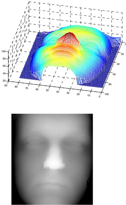
**Fig 1** Mesh plot of the range image (top) and gray level image plot of range data (bottom)
