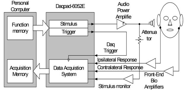
**Figure 2. Schematic layout of the functional components in the instrument design.**
