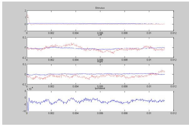
**Figure 4. Screen capture of the operator interface. From top to bottom: Stimulus monitor, Left AEP, Right AEP and Averaged Ipsilateral AEP.**
