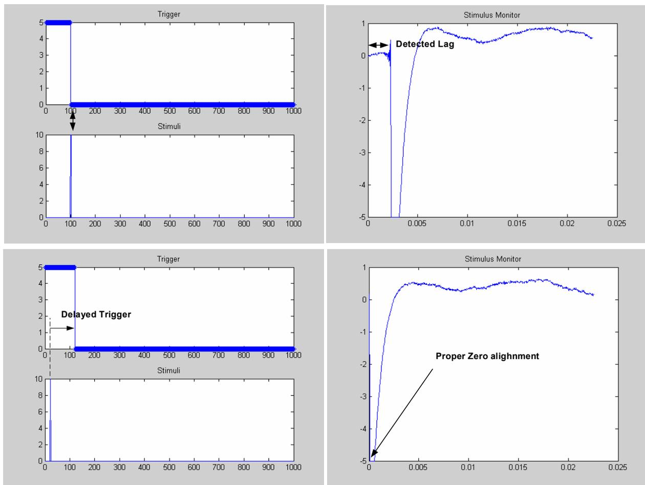
**Figure 3. Calibration method for lag detection and zero alignment. Top: pre-calibration, Bottom: post-calibration**
