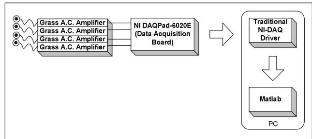
**Figure 2. Recording structure for EMG signals**
