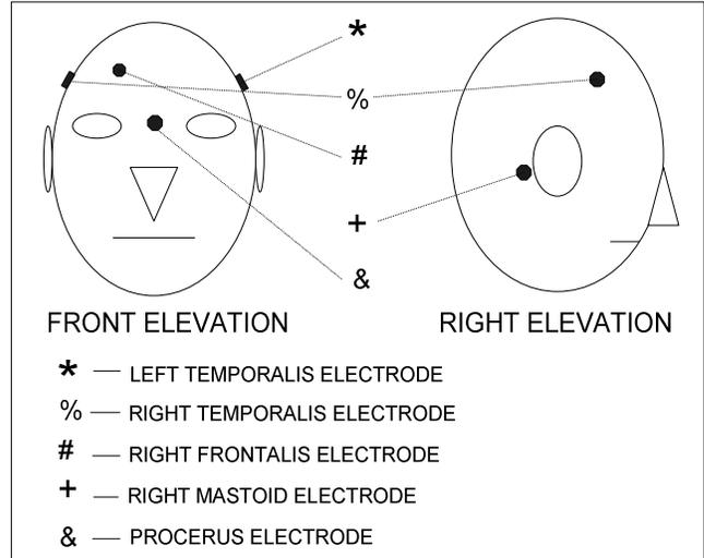
**Figure 1. Electrode placement diagram for EMG system**
