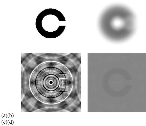
**Figure 1. Sequence of convolution and pre-compensation**
