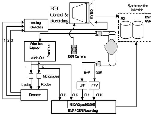
Figure 1: Instrumentation setup
