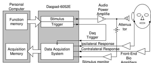
Figure 2. Schematic layout of the functional components in the instrument design.
