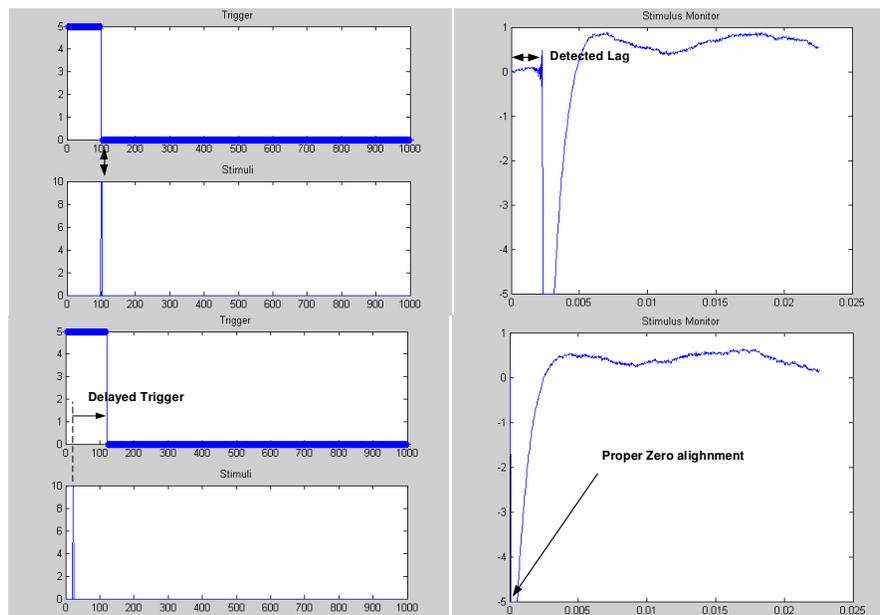
Figure 3. Calibration method for lag detection and zero alignment. Top: pre-calibration, Bottom: post-calibration.
