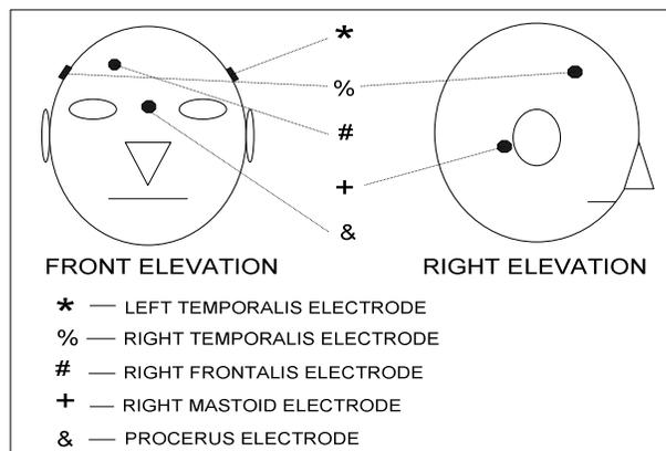
Figure. 2. Electrode placement diagram for the EMG system
