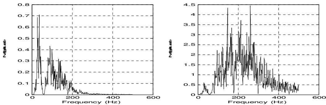
Figure 1. Spectra observed during a right frontalis contraction (left plot) and left temporalis contraction (right plot)
