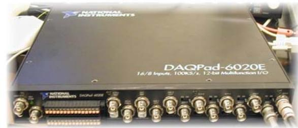
Figure 4: Multi-channel National Instruments DAQPad 6020E Analog-to-Digital Conversion System
