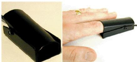
Figure 2: UFI Finger Clip Photoplethysmograph Model 1020FC
