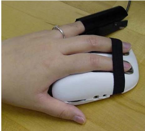
**Figure 1:** Galvanic Skin Resistance (GSR) sensor (white) and Photoplethysmography (PPG) sensor (black) used to measure the subject's Blood Volume Pulse (BVP) signal, shown as attached to the subject during the experiments.
