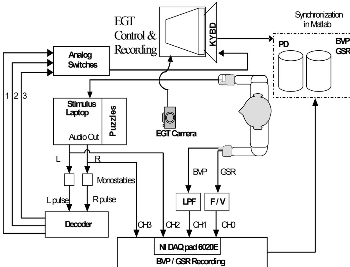
Figure 3: Instrumentation setup.
