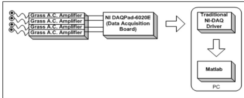
**Figure 2:** Recording structure for EMG signals
