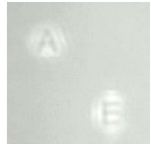
Fig. 4. A new precompensated image, adjusted for 4 mm, seen with the artificial eye at 4mm.
