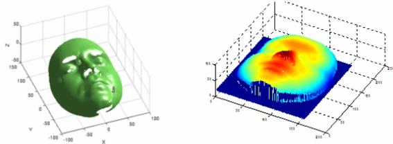
Figure 2 3D surface (left) and mesh plot of the converted range image (right)
