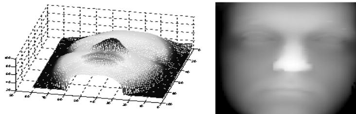
**Fig 2** Mesh plot of the range data (left) and gray level image of the range data (right)
