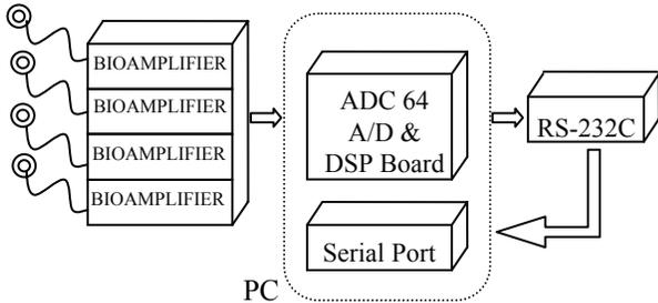
**Figure 3. Block diagram showing the functional blocks involved in implementing the EMG-based cursor control approach for real-time performance**
