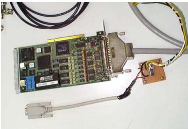
**Figure 4. Picture showing three key elements of the real-time implementation: the ADC64 board, the RS-232 driver and the connector to the serial port of the computer**
