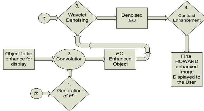
**Fig. 3.** Summary of the HOWARD algorithm. 1.  $H^1$  is generated using the desired threshold,  $th$ , and the user's unique wavefront aberration function given in the form of Zernike polynomials. 2. The Object to be enhanced for the user is convolved with  $H^1$ . 3. Wavelet denoising is applied to the  $EO$ , image to produce the denoised version of  $EO$ . 4. Then contrast enhancement is applied to yield the final, HOWARD enhanced image to be displayed to the user.
