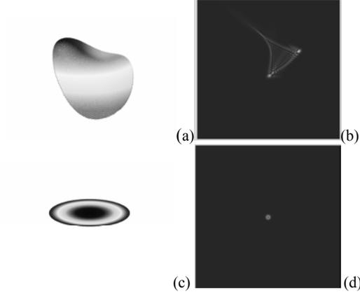
**Fig. 2.** Wavefront aberration (a,c) and Point Spread Function (b,d) for aberrated and ideal human eye, respectively.
