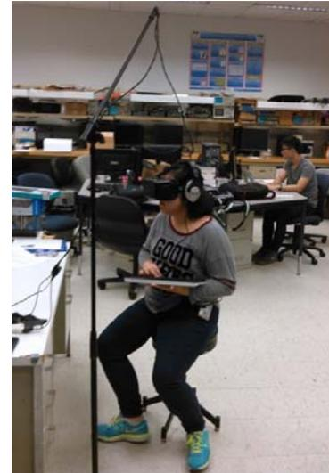
Figure 4: A subject performing virtual navigation. The visualization is performed with the Oculus Rift. The sound is delivered through stereo headphones and the subject advances or retrocedes by pressing arrow keys on the keyboard.
